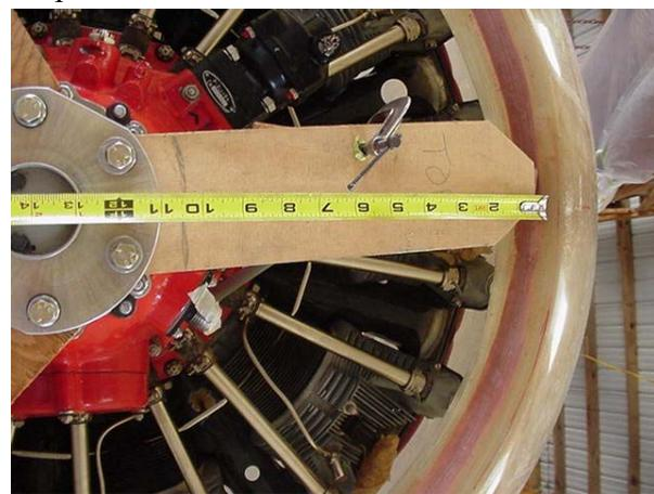
The cowl leading edge should not extend forward for the rear face of the prop flange. One side at the joint will be even with the rear face of the flange while the other will be back  $\frac{1}{2}$ " or so. This is do to the left thrust. Use wedges at the baffles to help center the cowl on the engine. The inner cuff should not contact the engine.
