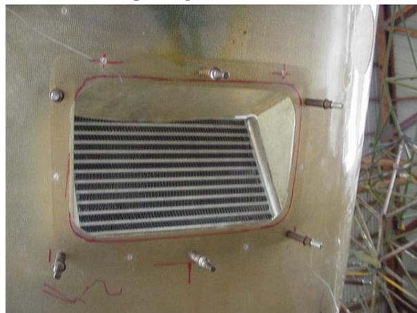
Locating scoop. On centerline at rear and must be aligned to look forward even though the cowl is off set.
