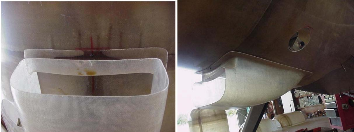
Following these steps, cut the remaining holes for exhaust, oil tank, air bottle access, intake drain, etc. Adjust these openings to fit your parts. We suggest that the oil and air doors and frames are made of .050" aluminum. Make sure you have 1/2" clearance around exhaust pipes and carb intake tube. The cap between the inner surface of the cowl and the baffles is to be sealed with a foam strip tie wrapped to the baffles. Do not operate the engine without this seal in place.
