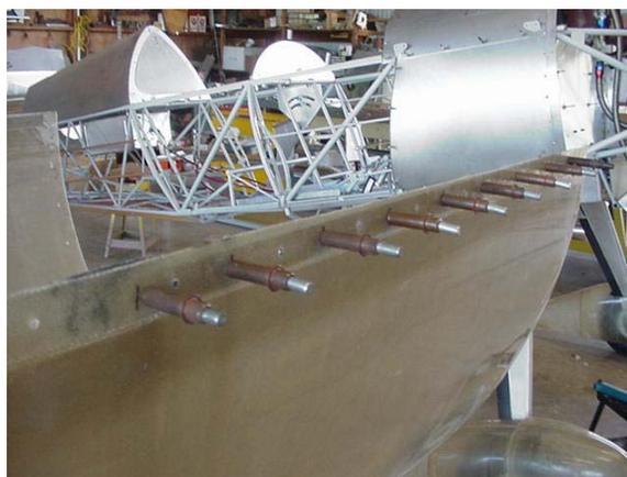
Cleco the strips in place. Note that 6 strips are used. From the inner cuff rear edge aft to the firewall each side, from the leading edge to the rear of the cuff on the outer joint, and the inner cuff. Strips are flush riveted 1 rivet between each nut plate.
