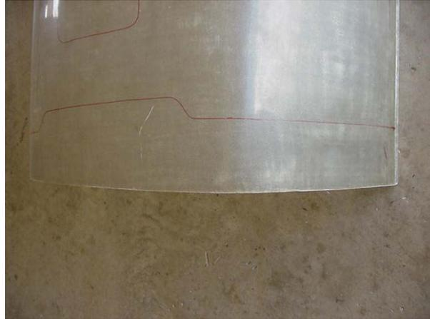
Find the center top of the upper cowl at the rear edge or at the scribe trim line. Sand the edges where the top and bottom cowl halves join on each side. Try for a very nice fit with 1/16" gap. Less than 1/16" gap at all joints will result in paint chipping later.
