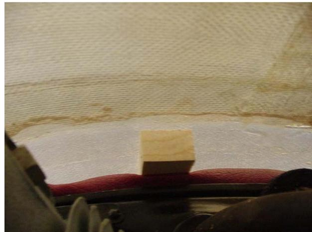
Hold the cowl halves together with straps while drilling the holes at the side joints and firewall that match the nut plates already in the firewall strip. Screw spacing is 3-3.5" as needed.
