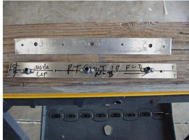
Fit oil cooler duct such that it lines up with the cooler and the opening. Screw holes as shown.
