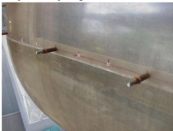
The screw locations at the joint in the inner cuff are located at 3", 6", 9" from the leading edge of the cowl. .032" x 3/4" wide Aluminum strips are used to reinforce the joints in the cowl. 10-32 nut plates are riveted to the strips and then the strips are epoxied and riveted into the cowl as the following photos show.
