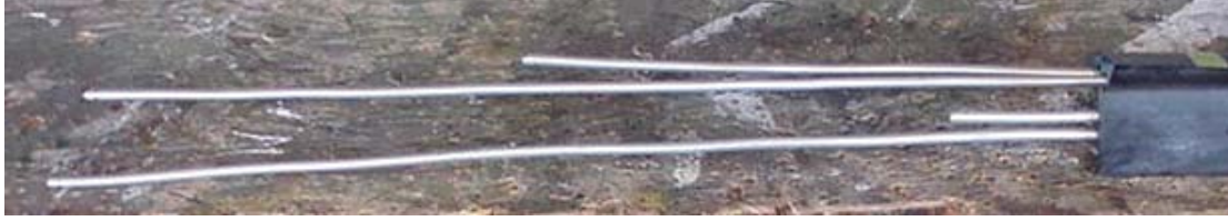
Alum brake and vent lines installed in fairing material
