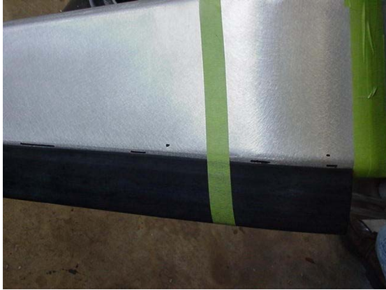
Fairing temporarily installed on gear spring with tape. Mark location on leg.
