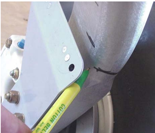
Lower end trim point even with top of wheel pant bracket. Upper trim point.
