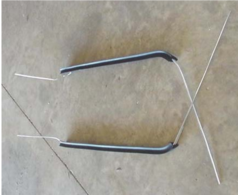
gear fairing shaped with brake and vent lines installed
